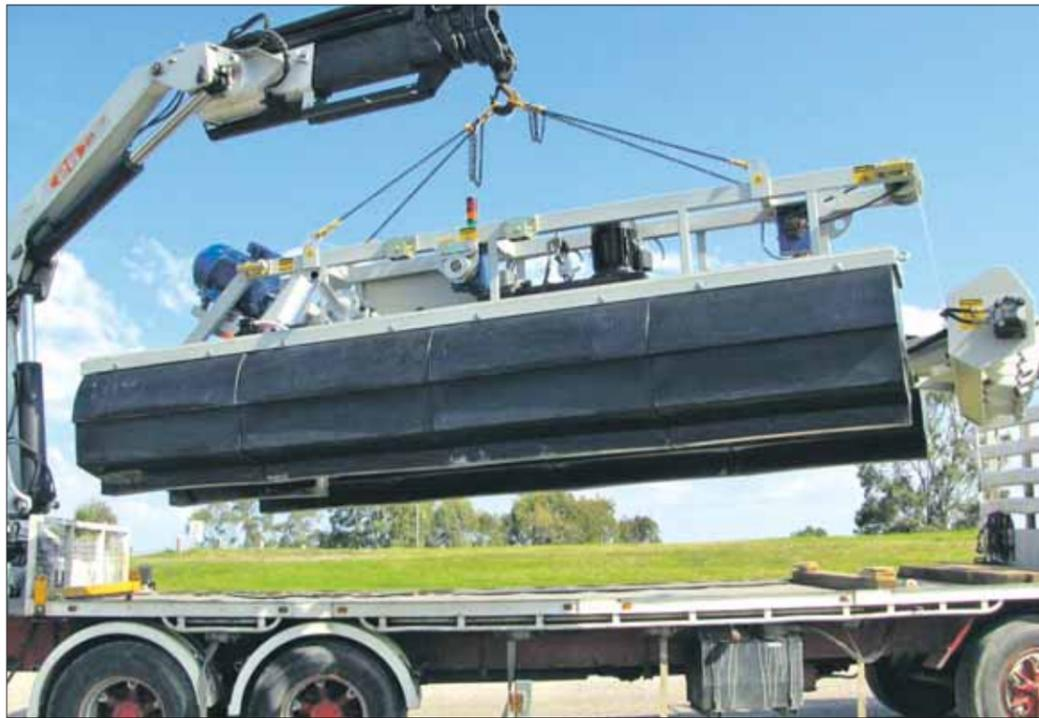
**Light and compact:** The new CatFish mini suction dredge is remotely controlled and unmanned.
